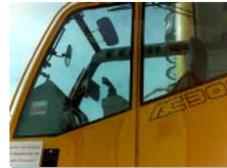
20° tiltable superstructure cab
