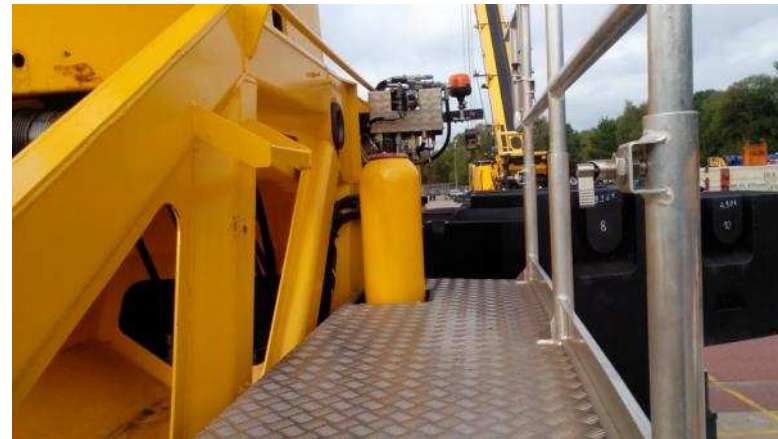
Guard rail around the superstructure
